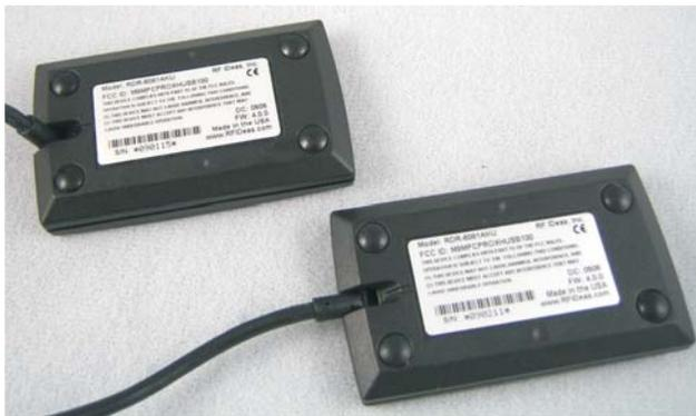
Part numbers with RDR only: Articulating cable allows for flush mount or desktop usage. Dimples on rear accept self-taping screws for
